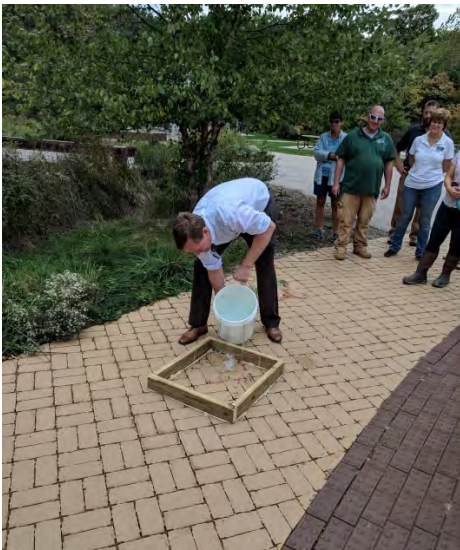
FIGURE 1 STANDARD TEST FRAME FOR INFILTRATION TEST
