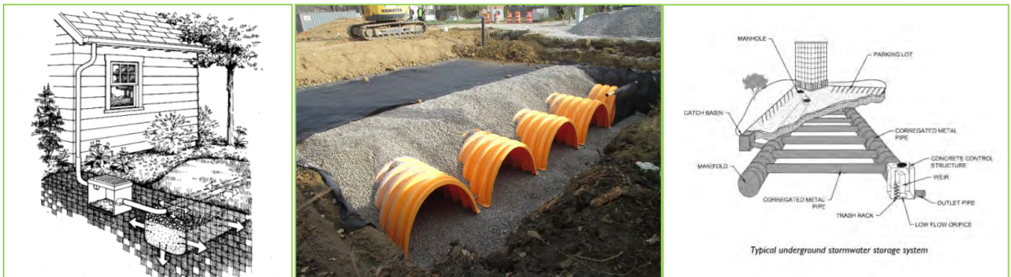
FIGURE 5-1 TYPICAL UNDERGROUND STORAGE CHAMBER CONFIGURATIONS
