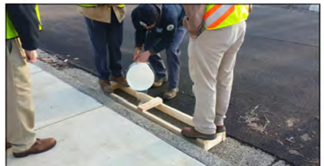
FIGURE 4 ALTERNATE TEST FRAME FOR INFILTRATION TEST
